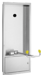
Pull-Down Eye Wash Recessed, wall mounted (4" deep), pull-down eye wash safety station. Stainless steel. 1/2" NPT. Barrier free. Cat. No. 93968
