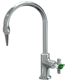
Single Service Gooseneck Faucet Single water, 6" swivel gooseneck. 3/8" NPT. Cat. No. 50015 with vacuum breaker Cat. No. 50010
