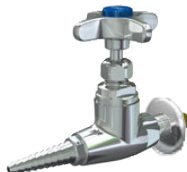
Single Keycock Single flange mounted needle valve, keycock with integral flange and shank connection. Epoxy coated brass. 3/8" NPT with lock nut. Single Cat. No. 50025 Double Cat. No. 50125
